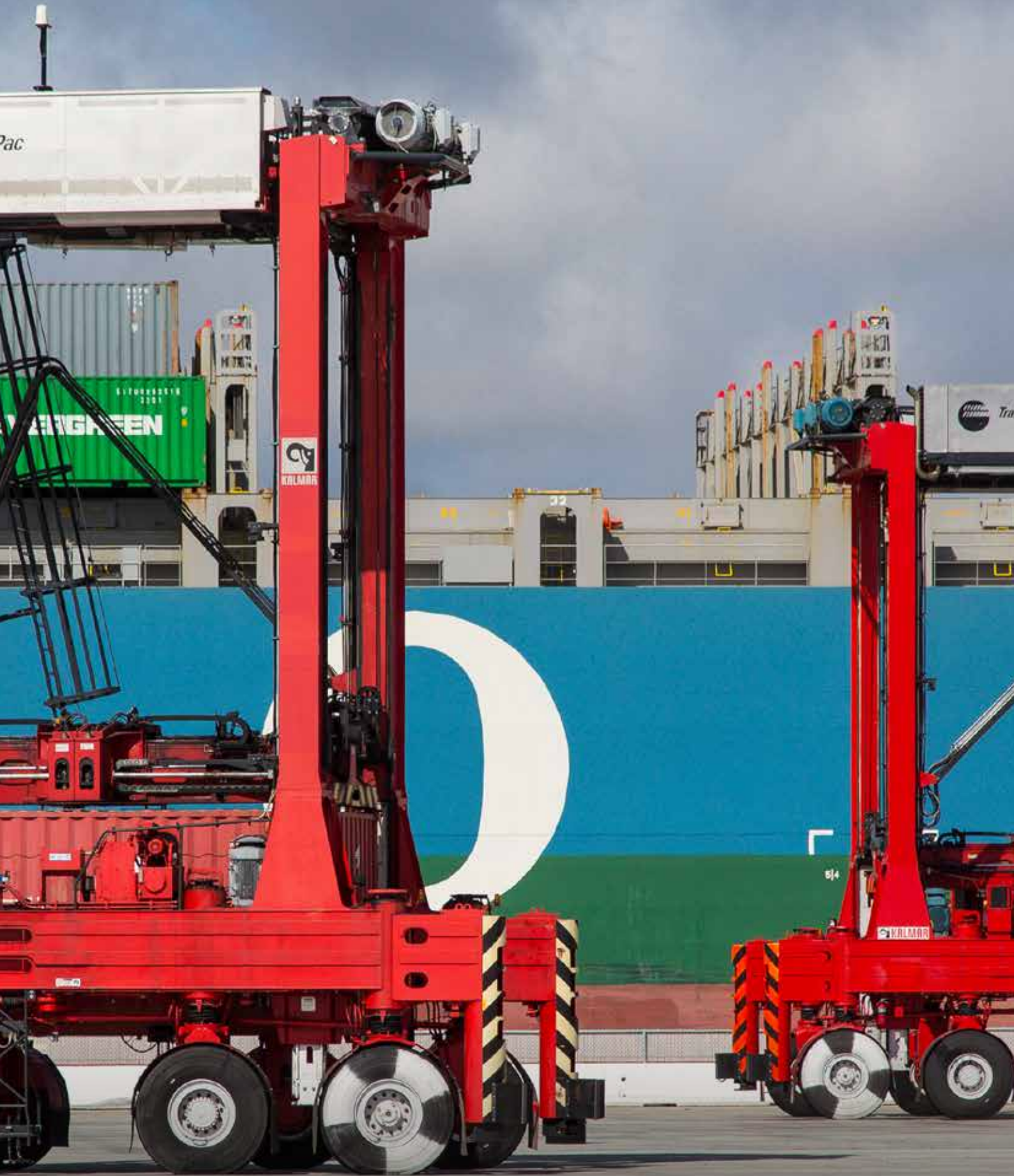
Fully automated vehicles moving containers at the port of Los Angeles. © Tim Rue/Bloomberg/Getty Images
